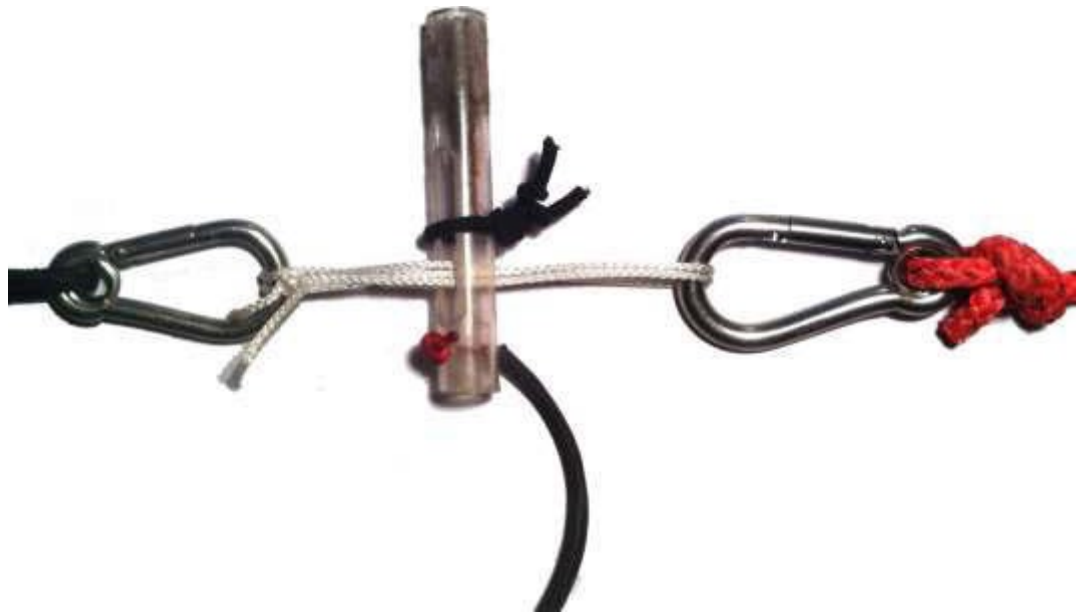
Figure 3 - Link Knife. In this photo, the o-ring has been replaced by a bungie cord.
